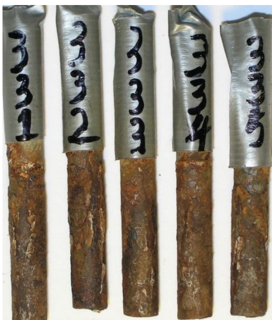
Figure D-4: Raw image of steel bars in MMA-treated HCP specimens of Group 4 (HCHV).
