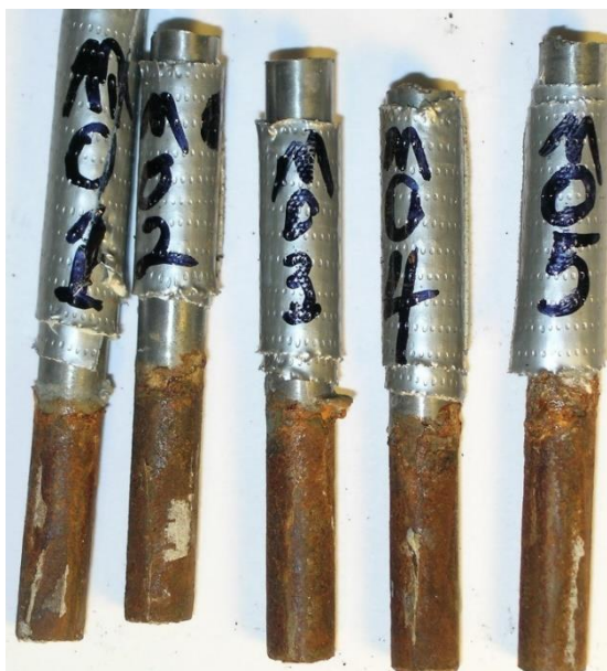
Figure D-6: Raw image of steel bars in MMA-treated HCP specimens of Group 6 (Y-MMA).
