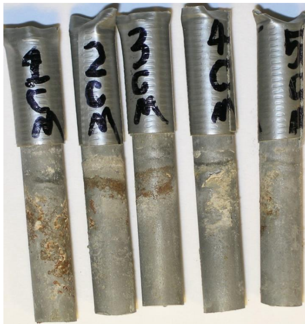
Figure D-2: Raw image of steel bars in MMA-treated HCP specimens of Group 2 (LCLV).
