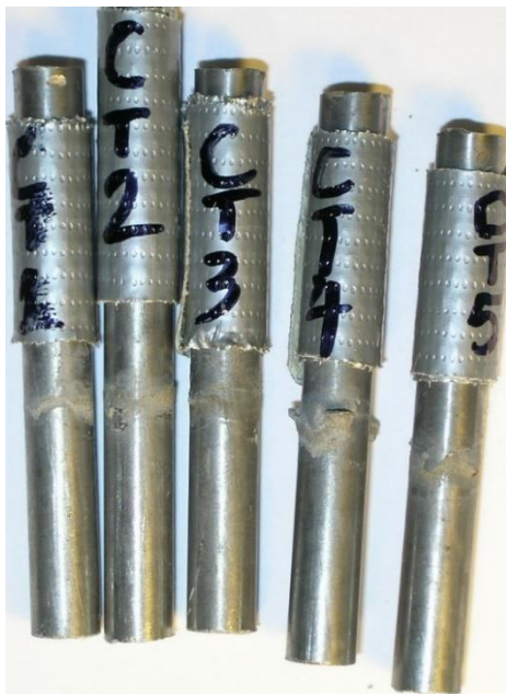
Figure D-7: Raw image of steel bars in control HCP specimens of Group 7 (Y-Control).
