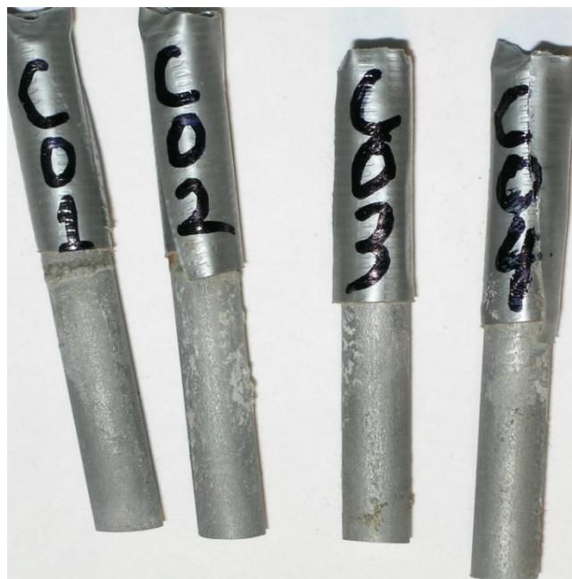
Figure D-5: Raw image of steel bars in control HCP specimens of Group 5 (O-Control).
