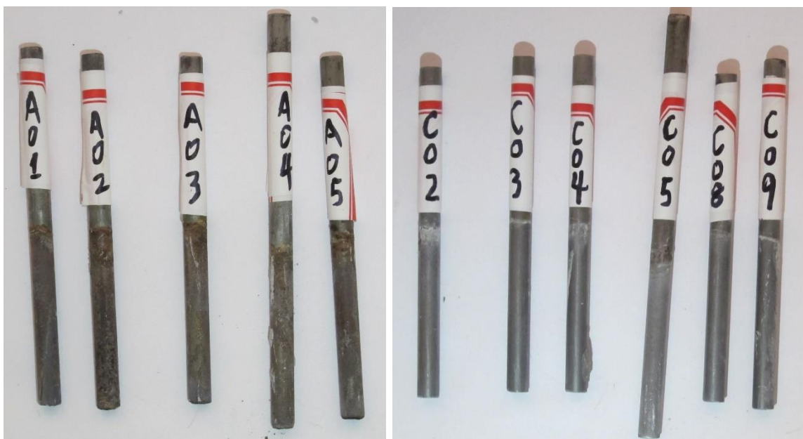
Figure 4-38: Comparison of bars from the MMA-treated group (Left) and the control group (Right) in Trial 3. The steel bars in the MMA-treated HCP exhibited a brown corroded coating (Left). The target corrosion potential for treatment was maintained at +0.57 V. Trials 1, 2, and 4 exhibited no sign of corrosion on the MMA-treated bars.
