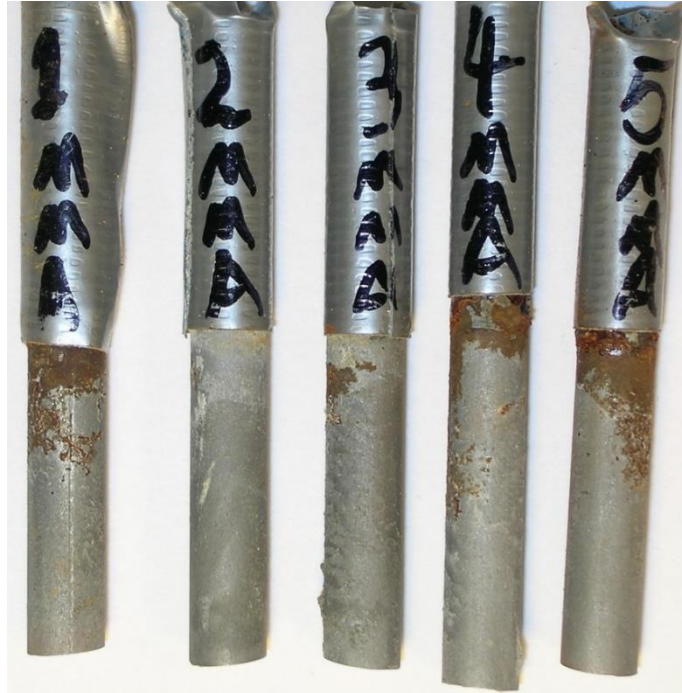
Figure D-1: Raw image of steel bars in MMA-treated HCP specimens of Group 1 (O-MMA).
