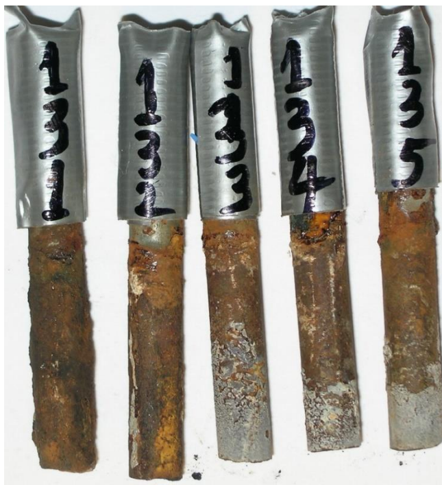
Figure D-3: Raw image of steel bars in MMA-treated HCP specimens of Group 3 (LCHV).
