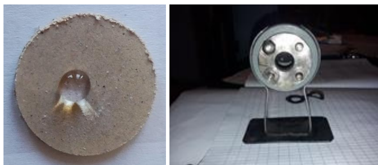
Figure 1. Hydrophobicity testing: a) water drop test and b) real conditions test.
