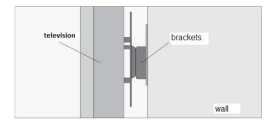
Bring the plasma or LCD with bracket installed to the other piece that is already fixed to the wall.
