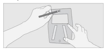
In the previously determined location that will provide support to the wall; mark where the holes will be made. With masonry bit to drill the holes at the marks.
