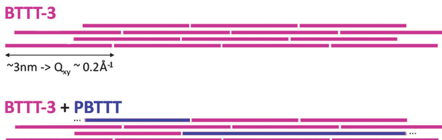
Fig. 4 Illustration of the proposed mixing of BTTT-3 and PBTTT chains within crystallites.
