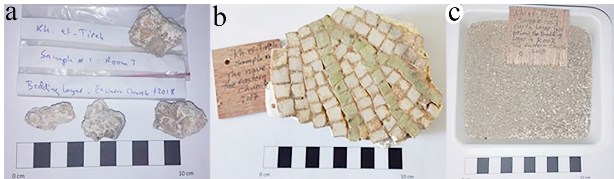
FIG. 10. Samples studied: (a) Sample # 1 consisting of several fragments of the mosaic from Room # 3 of the Eastern Church taken in 2018; (b) sample # 2 consisting of a mosaic fragment taken from the nave of nave of the Easter Church in 2017; (c) sample #3, taken from an earth layer found just below the bedding layer in Room # 3 of the Eastern Church.
