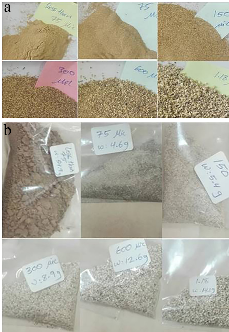
FIG. 13. Particle size distribution of the mosaic fill material: a) after screening of dry sample; b) after screening of wet sample.
