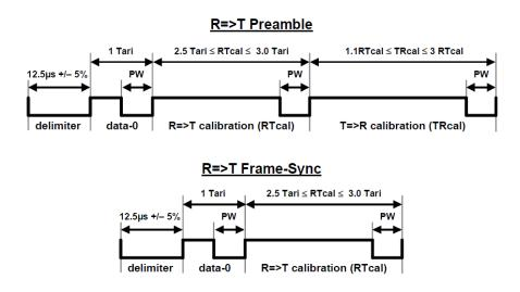
Figure 2.6: Reader to tag Preamble and Frame-Sync [2].
