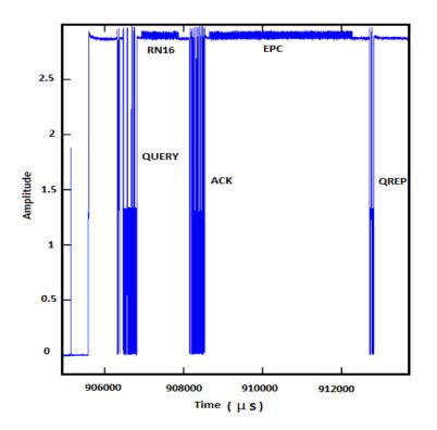
Figure 4.3: Gen2 RFID Reader Full Communication Cycle.
