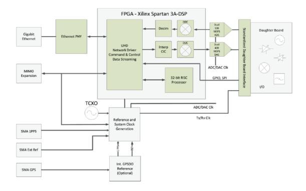
Figure 3.4: USRP N210 Hardware Architecture [7].
