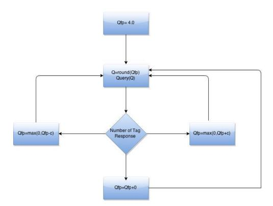
Figure 2.12: Q-algorithm used by EPC Gen-2.
