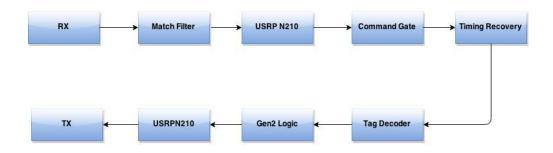
Figure 3.6: Gen2 RFID Reader System Architecture.
