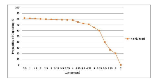
Figure 4.7: Probability of Capturing Versus Reading Distance.
