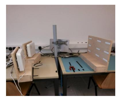
Figure 4.9: System Setup with commercial RFID Tags.
