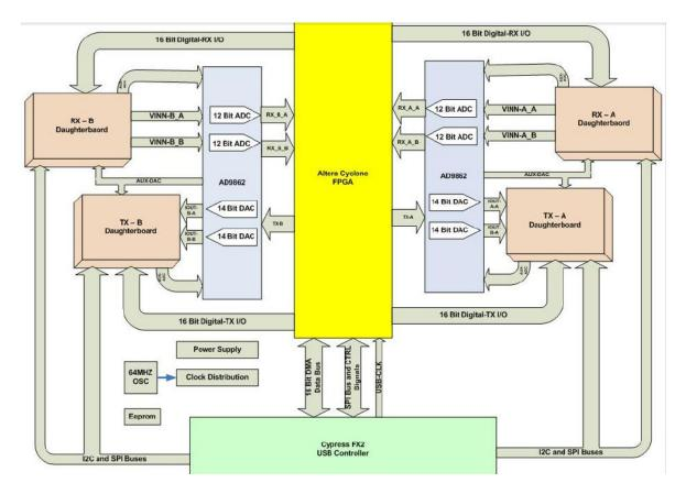
Figure 3.3: USRP1 Hardware Architecture [46].
