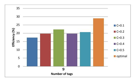
number of tags (optimal case of Q-algorithm) the efficiency increased to reach 29%. The best value of parameter C is equal to 0.3 where the maximum efficiency is about 23%.
