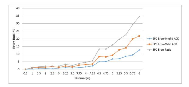
Figure 4.5: Error Ratio versus Reading Distance.
