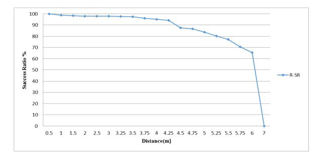
Figure 4.4: Success Reading Ratio versus Reading Distance.
