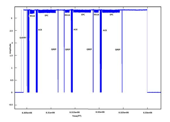
Figure 4.8: Communication Cycle between Our Reader and Tags Based on DFSA.
