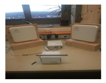
Figure 4.2: Two circular antennas are connected to USRP N210 which works as a reader.
