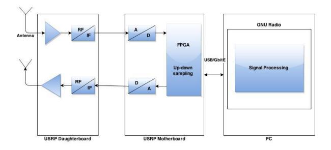
Figure 3.1: Software-Defined Radio Block Diagram.
