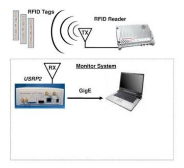
Figure 1.1: Monitor System Diagram [11].
