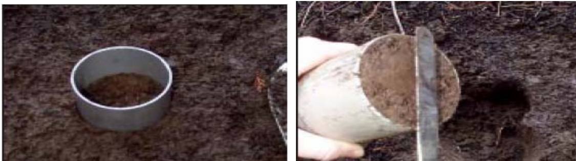
Figure ( 1.2 ): The cylinder of core method before inserting in the soil and after.
