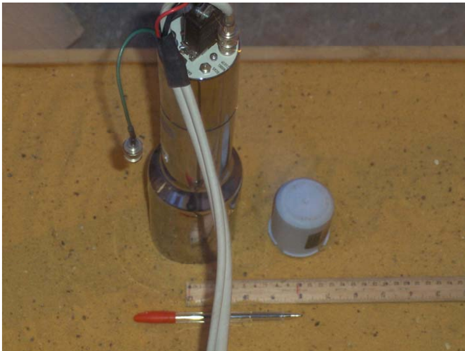
Figure (4.4): Gamma ray backscattering spectroscopy system with detector placed with face down and the shielded source placed 10 cm away from the detector.
