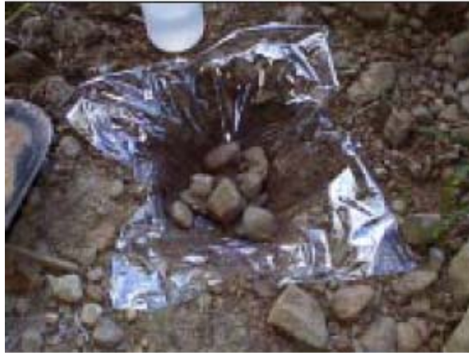
Figure (1.4): A hole lined by the plastic and fixed by rocks to fill with water for volume measurement in excavation method.
