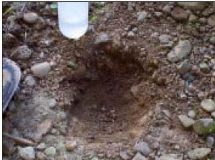
Figure (1.3): A hole digging in purpose to measure soil bulk density in excavation method.
