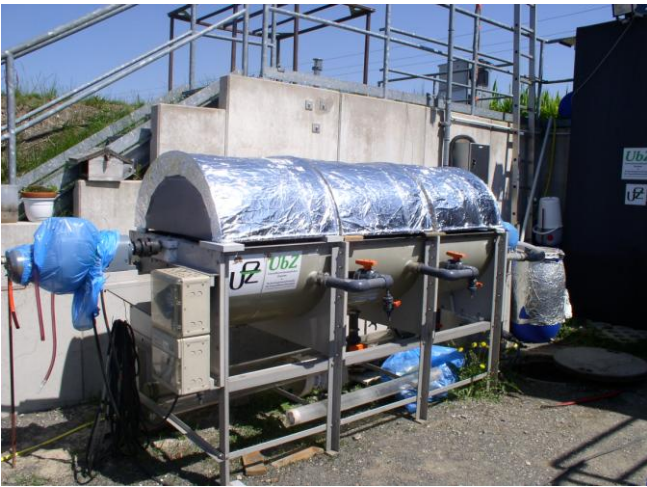
Photo A3: Covering the RBC by aluminum papers to reduce the effect of weather on the active biofilm which becomes attached to the disc surfaces
