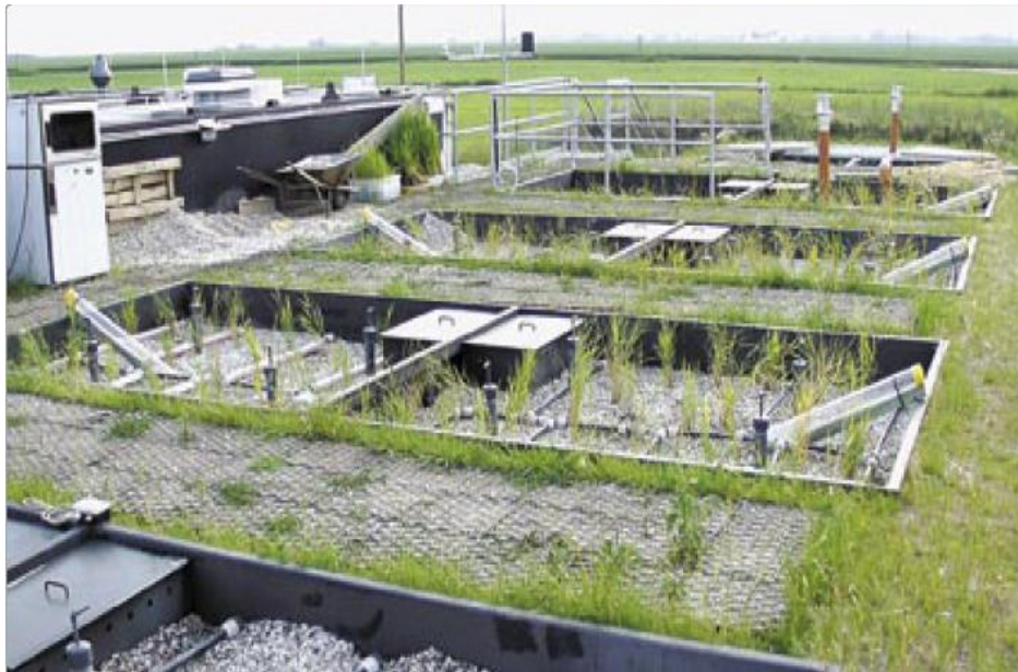
Photo 2.1: Phragmites australis reeds planted with a density of six balls per square meter.
