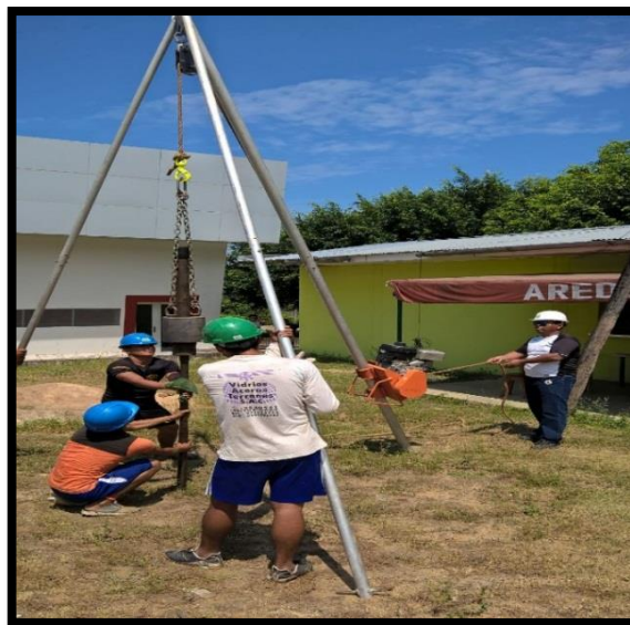
Foto 4: Standard Penetration Test. (SPT)
