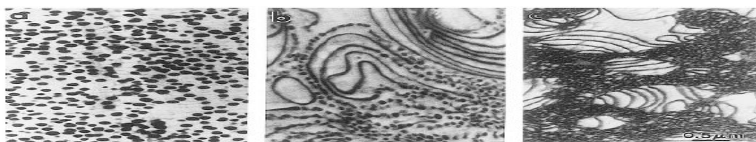
Fig.1.10.: Transmission electron micrographs of (a) the L1 (micellar) phase, (b) the asymmetric L3 (vesicular) phase, and (c) coexisting LR (swollen lamellar) and symmetric L3 (sponge) phases in blends with copolymers possessing 20, 30 and 40 wt % styrene/isoprene midblock, respectively. Note that the morphology depends strongly on copolymer architecture in these blends of equal composition ** .
