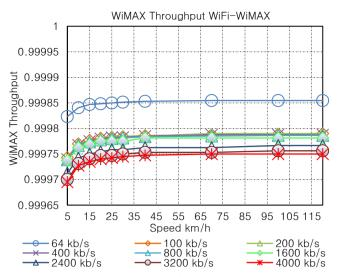
Fig. 3. Normalized throughput measured between media server and WiMAX interface on the mobile node for different bit rates in WiFi to WiMAX scenario.
