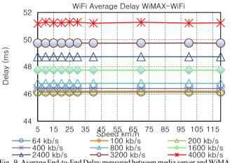
Fig. 9. Average End-to-End Delay measured between media server and WiMAX interface of the mobile node for different bit rates.
