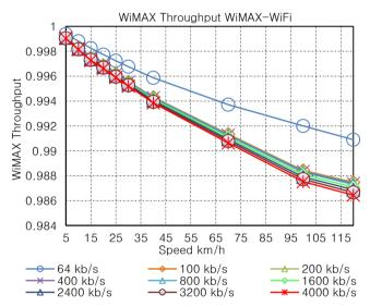
Fig. 4. Normalized throughput measured between media server and WiMAX interface on the mobile node for different bit rates in WiMAX to WiFi scenario.
