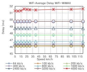
Fig. 6. Average End-to-End Delay measured between media server and WiFi Interface of the mobile node for different bit rates.
