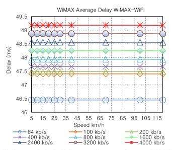
Fig. 8. Average End-to-End Delay measured between media server and WiMAX interface of the mobile node for different bit rates.
