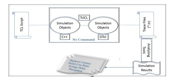
Figure 3.2: NS-2 architecture and simulation process.
