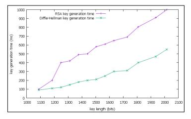
Figure2.7: Comparison between RSA and Diffie-Hellman Key Generation
