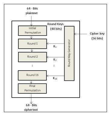
Figure 2.3: DES encryption process [29]
