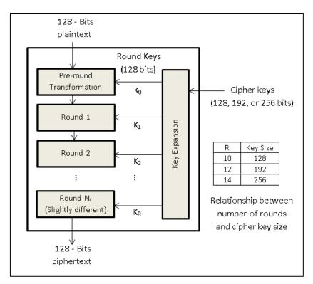
Figure 2.2: AES encryption process [29]
