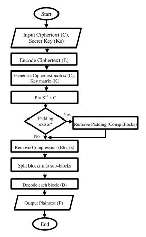
Figure 4.4: Decryption process flow chart
