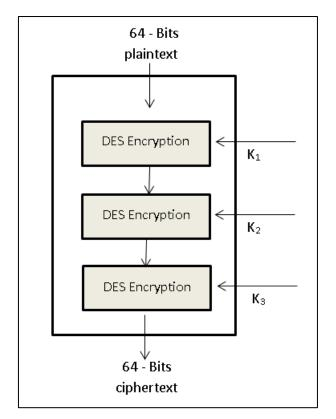
Figure 2.4: Triple DES encryption process [29]
