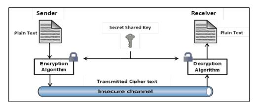
Figure 2.1: A simplified model for the symmetric encryption
