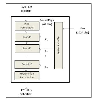
Figure 2.5: Blowfish encryption process [29]
