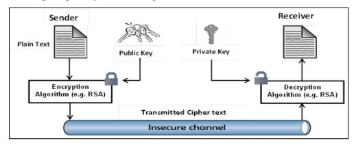
Figure 2.6: A simplified model for asymmetric encryption
