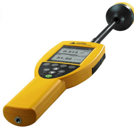
Figure 3.1 - NBM-550 Narda Broadband Field Meter
