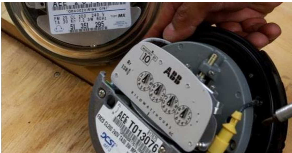
Ilustración 68 Medidores eléctricos hackeados. Tomado de Ireland Elizabeth, "Puerto Rico smart meters believed to have been hacked – and such hacks likely to spread | Metering.com" [205]
