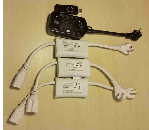
Fig. 1 – Devices used in the network under study. From top to bottom, this includes an Aeon USB ZStick2, a GE Outdoor Switch, and three Aeon Appliance Switches.
