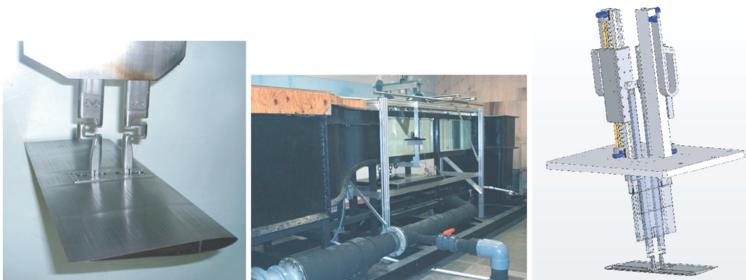
Figure 3. SD7003 airfoil installed in HFWT test section, with plunge rods in position prior to a run (left); Horizontal Free-surface Water Tunnel (middle); and schematic of pitch/plunge rig and airfoil model (right).
