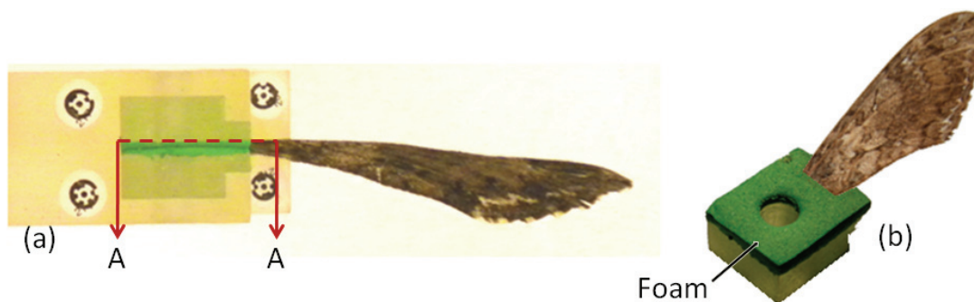
Figure 5. Side view of a clamped Manduca Sexta forewing (a), and the foam-lined clamp of cross-section A-A (b). The four symbols shown in (a) are reference points for future photo-modeling use.
