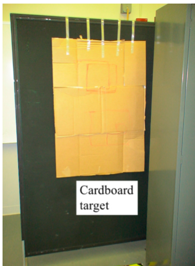
Figure 5.8: Cardboard target hung on a protective laser barrier. This target simulates the ground.
