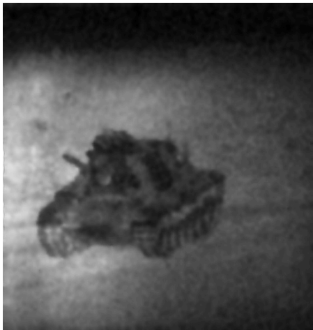
Figure 5.17: Image in Figure 5.16 denoised using HOD and a block size of six. Output PSNR = 33.17.
