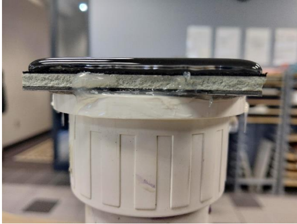
Figure 6.3.2: Water penetrating the seam and leaking to the back of the specimen
