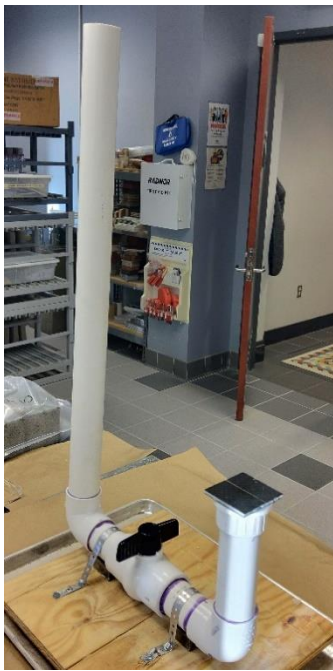
Figure 5.3.1: ASTM D4068 apparatus with specimen installed
