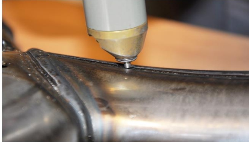
Figure 1.2: Ultrasonic peening process representation [3]
