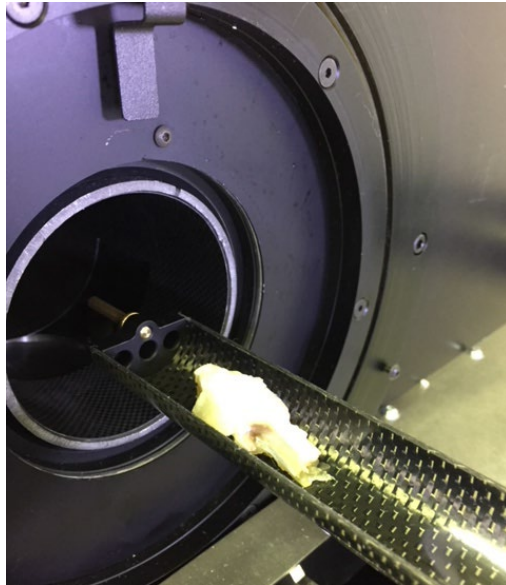
Figure 10: Dissected DHGP knee joint placement in Micro-CT bedding in preparation for imaging.
