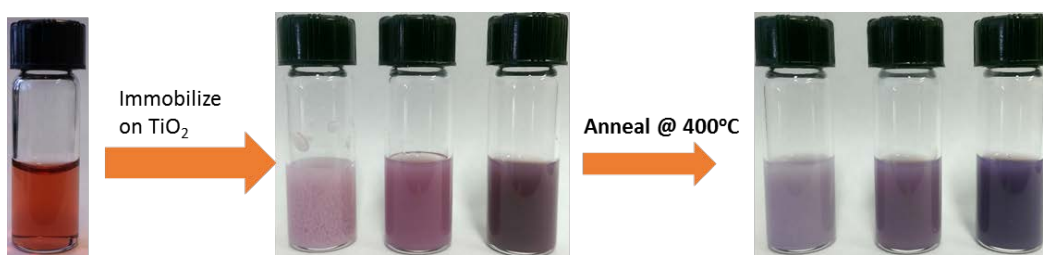
Figure 2.2. Immobilization of colloidal citrate-AuNP on titania and subsequent annealing at 400 °C. The growth of AuNP on titania during the annealing process is evident because of the color change from dark pink to purple.
