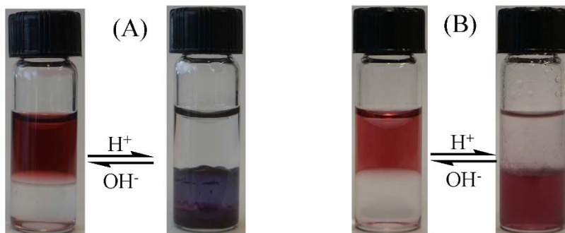
Figure 3.8. Control experiment to show that ODA facilitates the phase transfer of AuNP-MUA. (A) Without adding ODA, Photographs of glass vials containing aqueous solutions (top) of AuNP-MUA in contact with chloroform (bottom). The initial aqueous solution of the AuNP-MUA in the vial was red in colour with pH > 4.1 (left). By adding 0.1 M HCl, the pH of the AuNPs aqueous solution was gradually decreased below 4.1 (right). After vigorous shaking and storing for about 2 min, the thin film of aggregated AuNPs, formed at water/chloroform and chloroform/glass wall interfaces. Redispersion of the AuNPs back to the aqueous phase is observed by adjusting pH of aqueous medium > 4.1 by adding 0.1 M NaOH, and (B) With ODA, Photographs show the pH triggered reversible phase transfer of AuNP-MUA between water and CHCl_3 layers by switching the pH . The left side vial containing well dispersed AuNP-MUA in aqueous phase (top layer) at basic pH and right side vial containing AuNP-MUA transferred into CHCl_3 phase (bottom layer) after adding HCl and vigorous shaking and storing for about 2 min.
