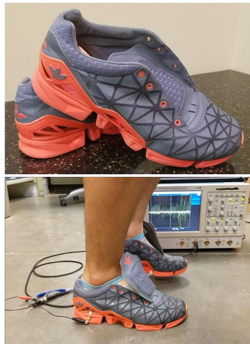
Figure 3.9 (a) A photo image of 3D printed shoe sole for hybrid structure based energy harvester, (b) demonstration of shoes application by hybrid structure based energy harvester with shoe sole.
