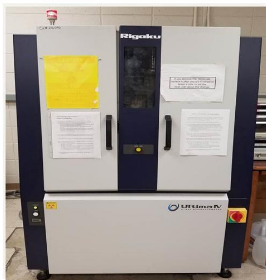
Figure 2.14 A photo image of X-ray diffraction (Model No.: Rigaku ULTIMA IV, Department of Chemistry in Clemson University)
