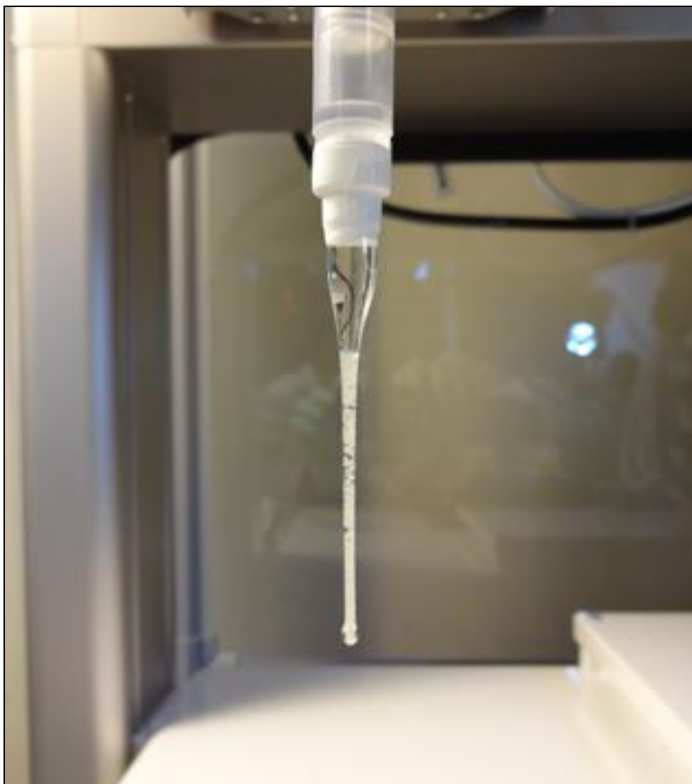
Figure 2.9: A picture showing the pasture pipette printing tip loaded with tissue spheroids for dispensing.
