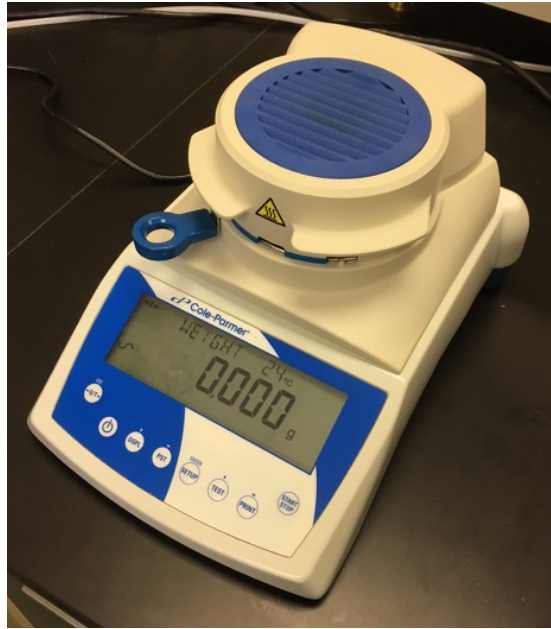
Figure 3.6: Moisture balance used to determine the percent moisture present in the corrugated specimens.
