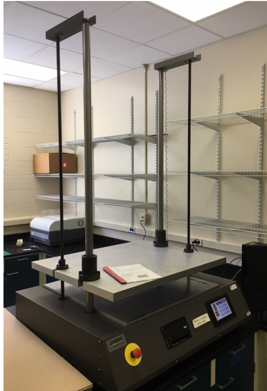
Figure 3.4: Lansmont Squeezer used for all compression testing.
