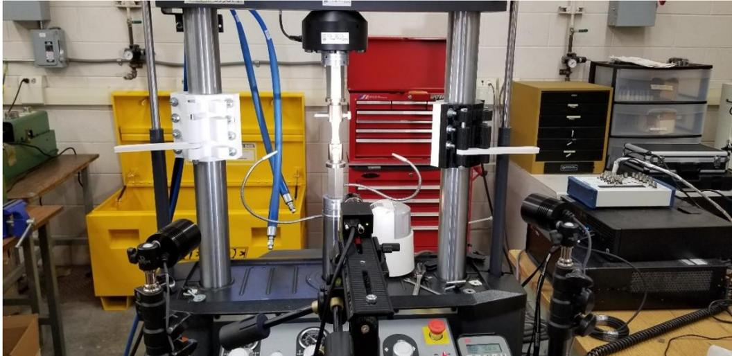
*Figure 5: Tubular tensile specimen experiment setup with MTS Landmark load Frame and digital image correlation*
