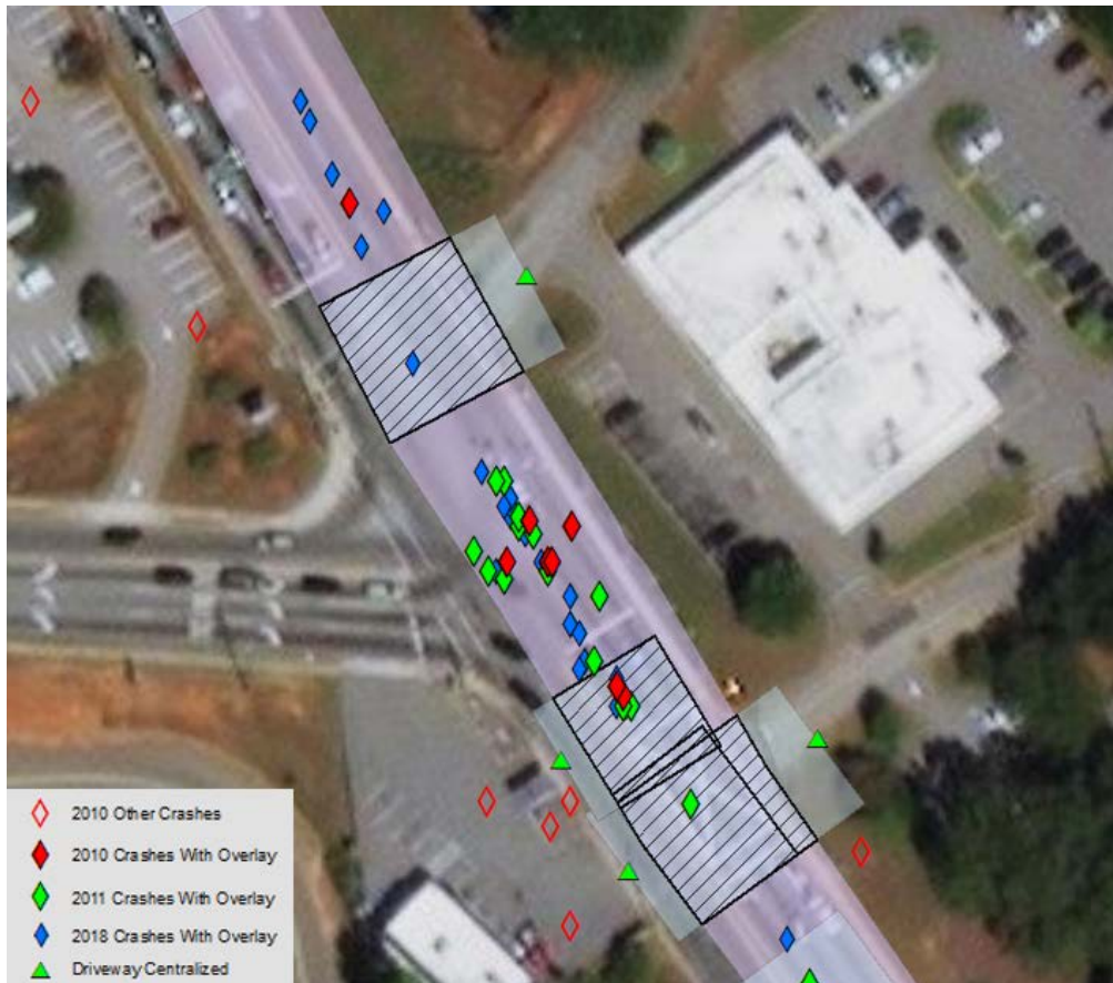
Figure 6: Driveway related crashes on US Highway 176 in Richland County, South Carolina. (image from Bing Maps)
