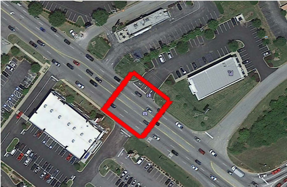
Figure 10: Crashes concentrated at a single driveway (Woodruff Road, Greenville)
