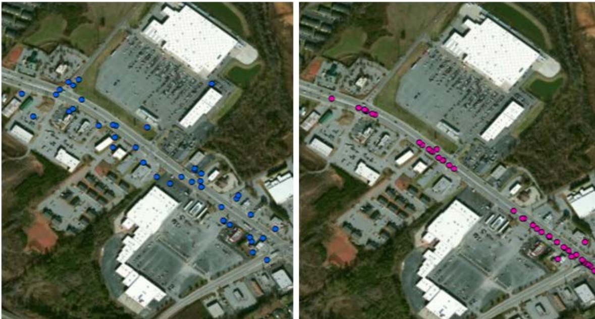
Figure 1: Rear-end and angle crashes on US 25 in Greenville, SC for 2010 (left) and 2012 (right) (images from Bing Maps)
