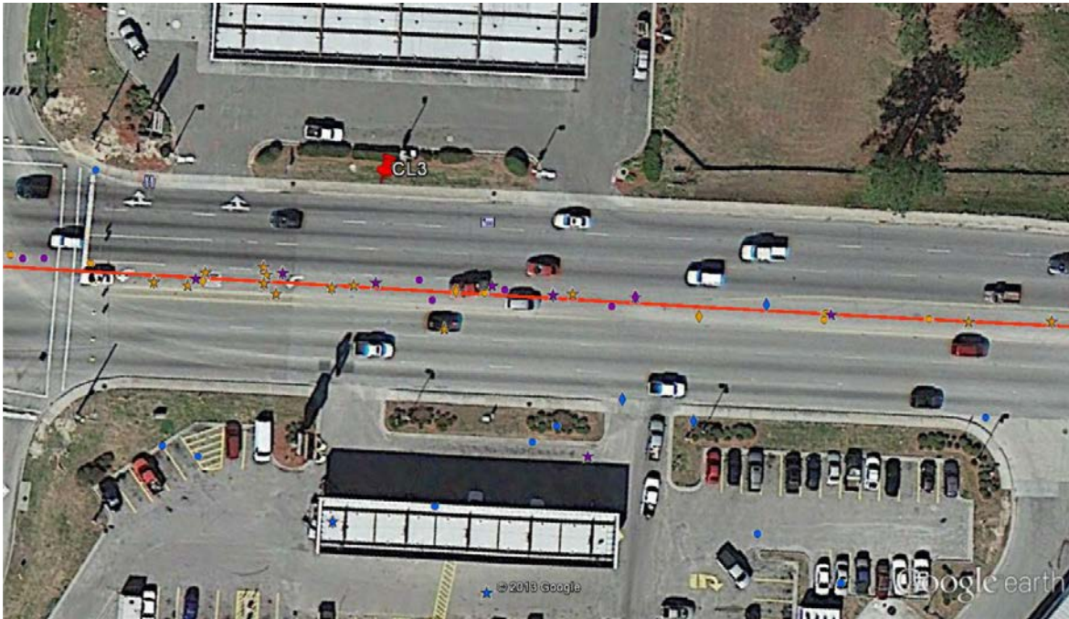
Figure 4 Crashes over a three-year period on US highway 17 in Berkeley County, SC *Coded driveway related crashes shown with stars. Note the proximity of the crashes relative to the left-turn bay. (Image from Google Earth)
