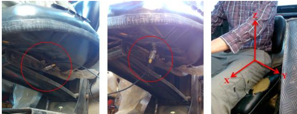
Figure 2. The position of vibration sensor in different directions of x, y and z
