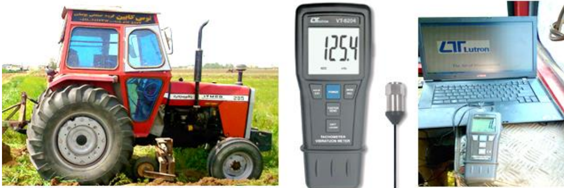
Figure 1. MF285 tractor equipped with the fifth wheel and vibration meter and laptop
