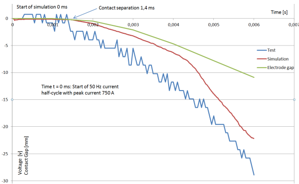
Figure 5. Experimental (blue) and simulated (red) arc voltages of gas arc vs. time. Measured contact gap (green) is input quantity for simulation.
