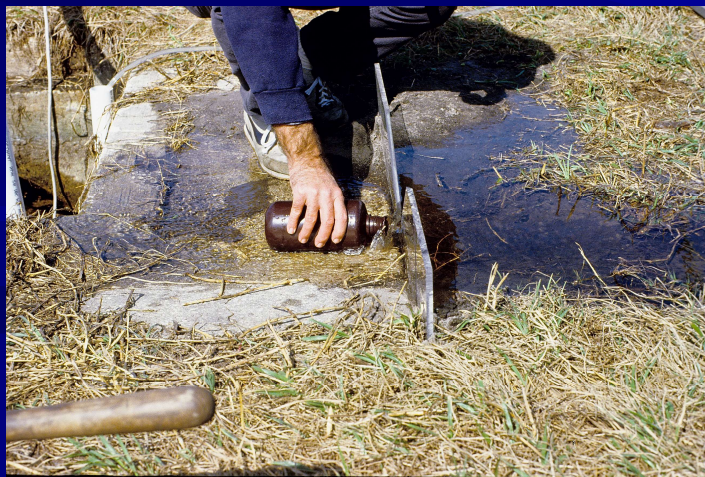
Water runs down swale and samples and flow data are collected
