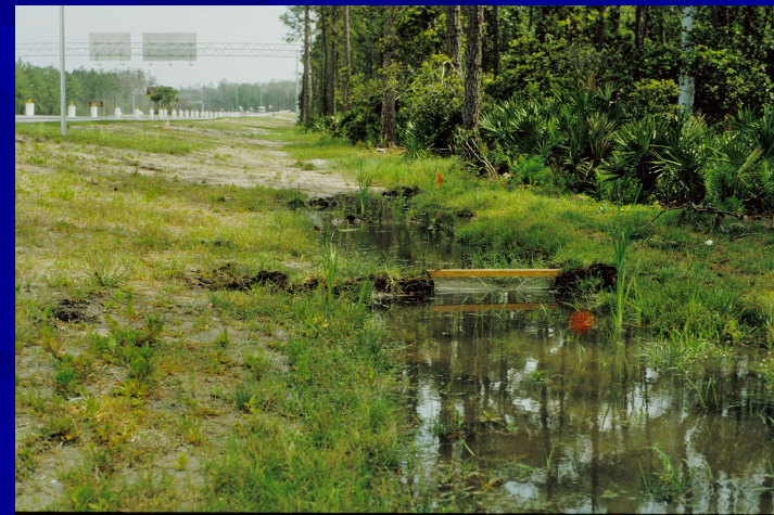
Water runs down swale and samples and flow data are collected
