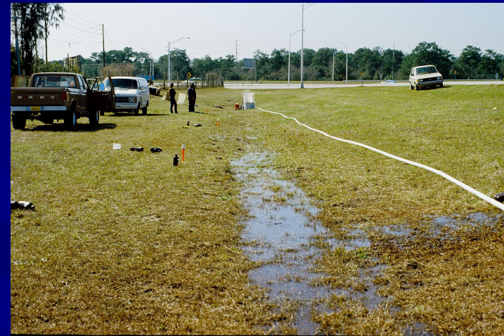
Water source is spiked with nutrients and metals and pumped into swale
