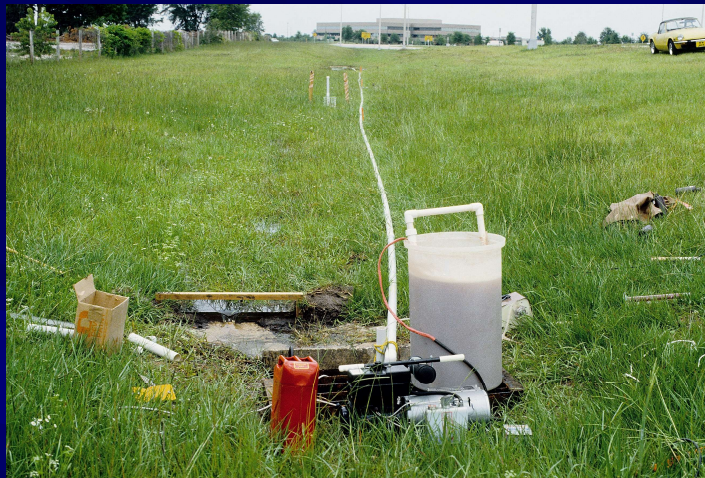
Water source is spiked with nutrients and metals and pumped into swale
