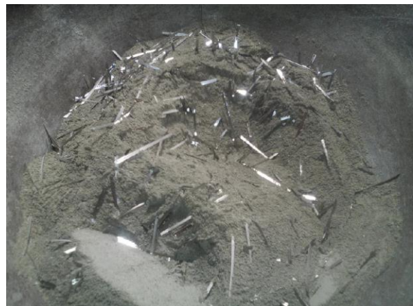
Figure 3. Amorphous fiber in the mixing stage with a cement-sand composition [1]
