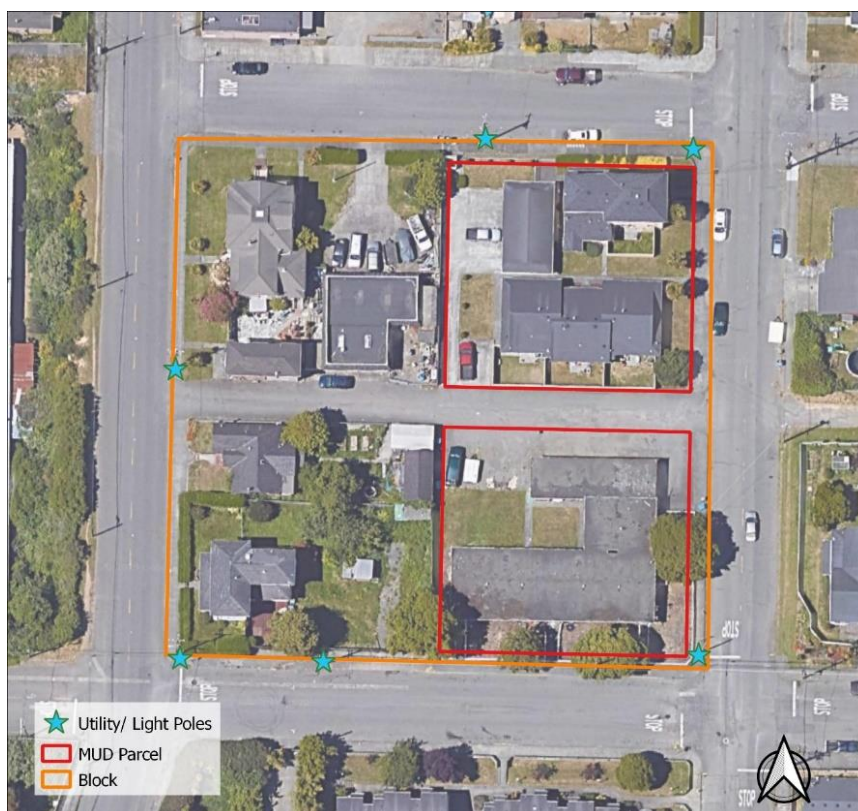
Figure 4-4 Example multi-unit dwelling (MUD) parcel without off-street parking availability and the identified light or utility poles located on the same side of the street on the block. Data sources: Google satellite image base map and Humboldt County parcel shapefile from Humboldt County GID department website.
