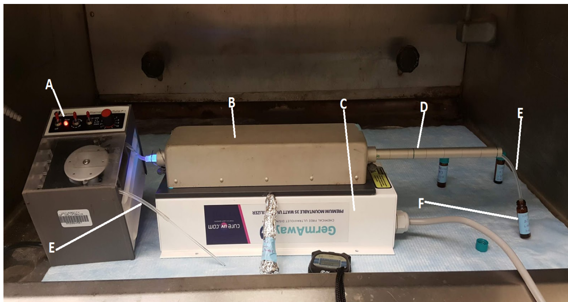
Figure 5: Test apparatus: A) Peristaltic pump B) Metal housing for quartz tube C) Low-pressure UV light D) Metal sheath E) Peristaltic tubing F) Amber collection vials
