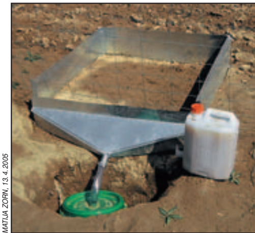
Figure 1: Erosion plot 1 on bare soil in a young olive grove and surface runoff captured in collecting container in the week between 7. 4. 2005 and 13. 4. 2005. The runoff was transferred to a 10-liter container.
