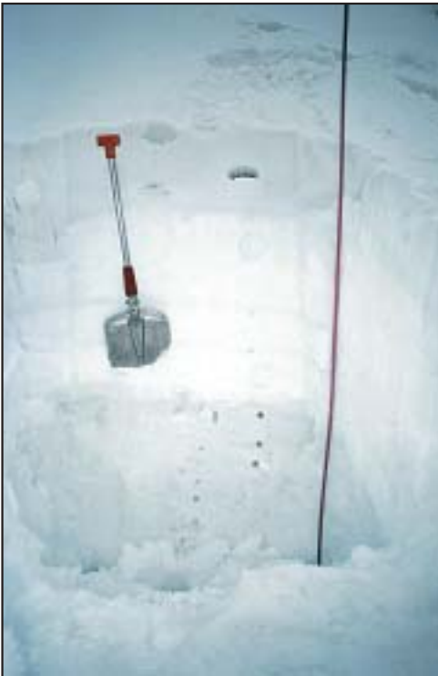
Figure 4: Snow profile, where all layers of snow cover can be identified. The avalanche shovel is 20 cm wide (photograph: Miha Pavšek).
