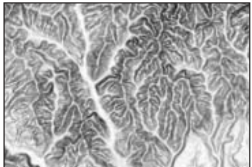
Figure 21: Surface slopes of DEM-25 with values between 0.00^\circ (lightest colour) and 32.80^\circ (darkest colour) for the Jerusalem area.
