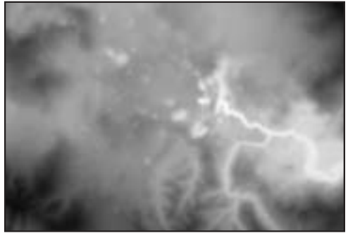
Figure 25: Surface heights of DEM-25 with values between 315.40 m (lightest colour) and 770.40 m (darkest colour) for the Škocjan area.
