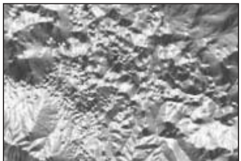
Figure 29: Surface aspects of DEM-25 with values between 0.00° (lightest colour) and 180.00° (darkest colour) for the Škocjan area.
