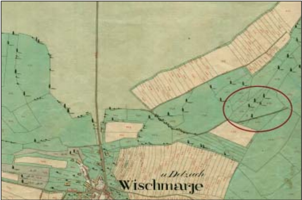
Figure 5: Section from the map of the Franziscan Cadastre for the cadastral municipality of Vižmarje, sheet L323A01, (Archives of the RS). The marked areas indicate meadows surrounded by boundaries that have survived completely unchanged to the present day.
