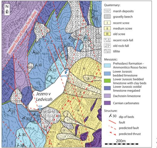
Fig. 4: Detailed geological map of the Jezero v Ledvicah lake area.
