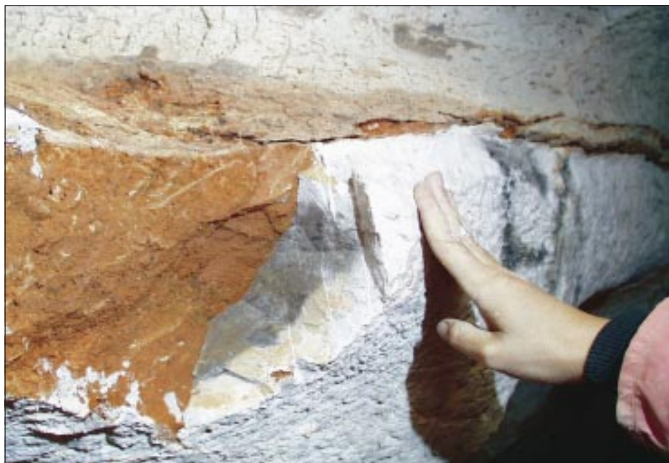
Fig. 1: Weathered limestone on the cave wall. Sl. 1: Preperel apnenec na steni jamskega rova.
