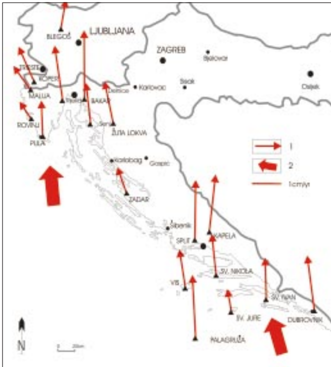
Fig. 10: Results of the GPS measurements (after Cigrovski-Detelić, 1998 and Altiner, 1999). 1-horizontal component of the movement velocity vector; 2-movement of the Adriatic microplate.
