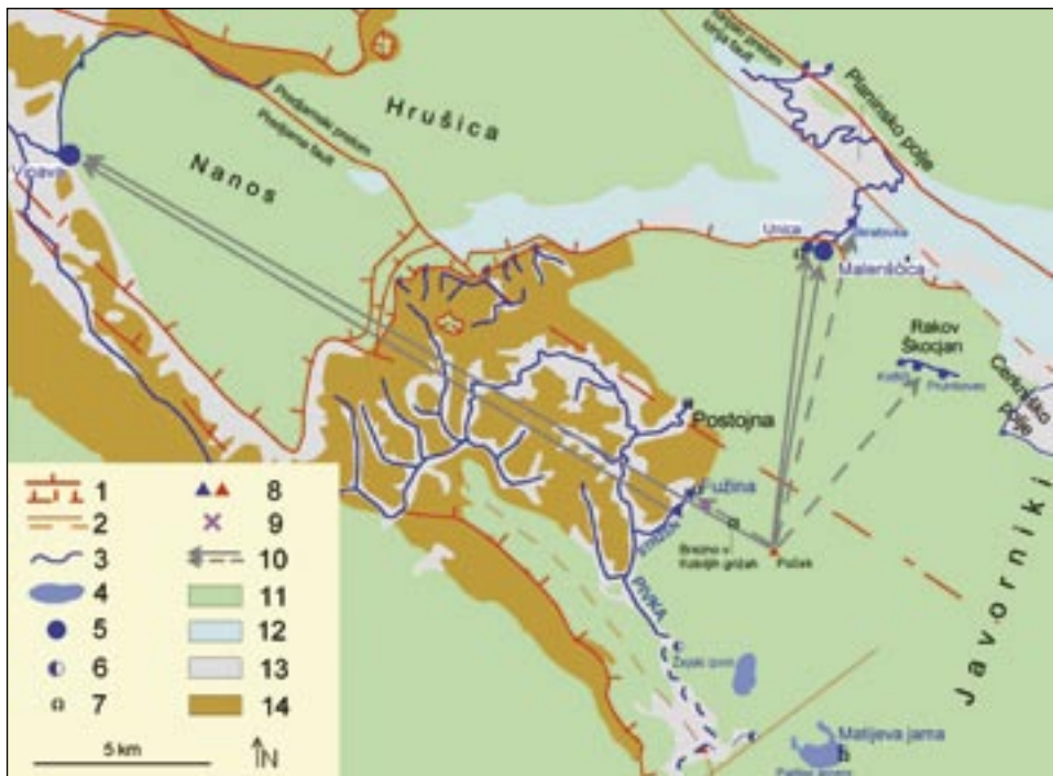
Figure 2: Hydrogeological map of the broader area of the landfill with the results of tracer tests (Legend: 1. Visible and covered thrust plane, 2. Visible and covered fault, 3. Surface stream, 4. Intermittent lake, 5. Permanent spring, 6. Intermittent spring, 7. Karst cave, 8. Ponor or injection point, 9. Landfill, 10. Main and secondary underground water connection, proved by tracer test, 11. Karst aquifer, 12. Fissured aquifer, 13. Porous aquifer, 14. Very low permeable rocks).
