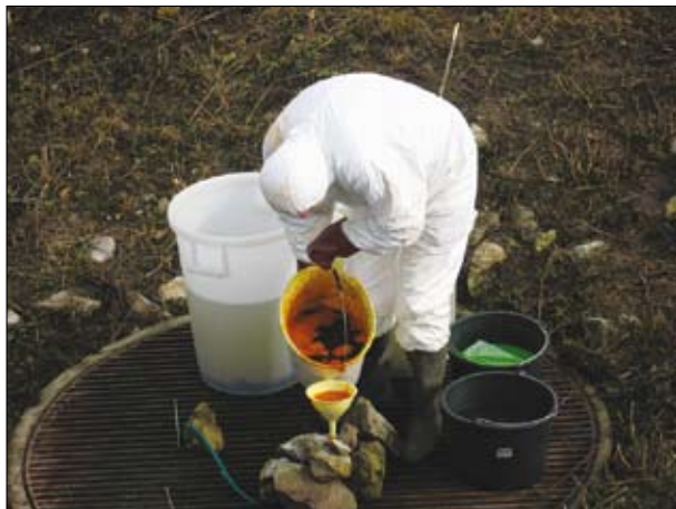
Fig. 5: Injection of uranine through the pipe into the fissure in the lateral wall of the ponor (foto: Janja Kogovšek).
