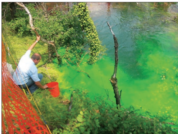
Fig. 6: Injection of the tracer fluorescent dye uranine (Photo: K. Mezga).
