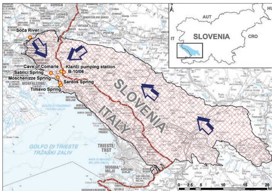
Fig. 1: The location of karst aquifer Brestovica, sampling points and direction of groundwater flow.
