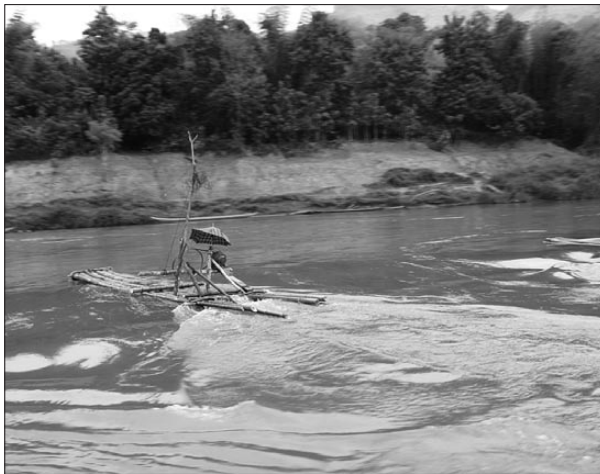
Fig. 20: In-stream micro hydro-electricity generation involving installation of small generators on moored rafts. Considerable potential exists for further such micro hydro generation to provide electrical energy for local communities (Photo: K. Kiernan).
