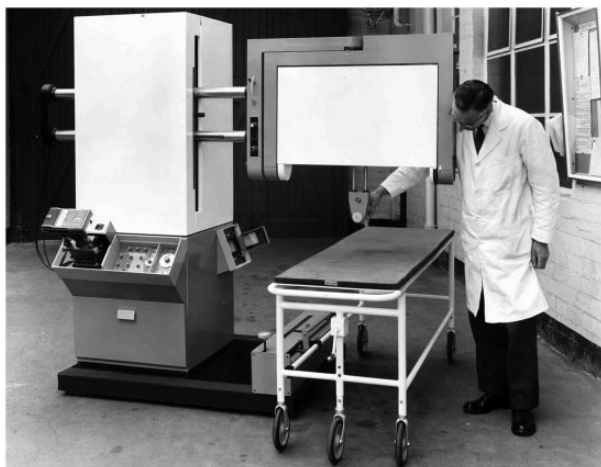
Figure 12. The first Disonograph, built at Kelvin Hughes at Hillington, c. 1964. Standing beside it, to add scale, is Arthur Johnson, one of the draughtsmen involved in the project. Photo reproduced by the kind permission of Dugald Cameron.
