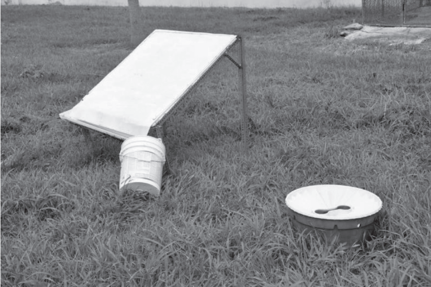
FIGURE 6. Planar dew condenser (condensing area = 1 \text{ m}^2 ) and Groassis Waterbox (condensing area approximately 0.16 \text{ m}^2 ) placed alongside each other for comparison of dew condensation.
