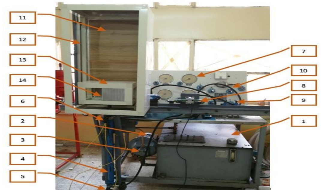
Fig. 5: Electro-hydraulic elevator system prototype; 1. Tank, 2. Electrical motor, 3. Constant displacement pump, 4. Hydraulic cylinder, 5&6. Pressure transducers, 7. Gauge pressure, 8. Proportional valve, 9. Pressure valve, 10. Flexible hose, 11. Elevator frame, 12. Distance sensor, 13. Cabin frame, 14. Cabin door
