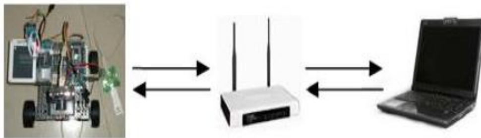
Figure 3. ARM9 wireless remote control overview
