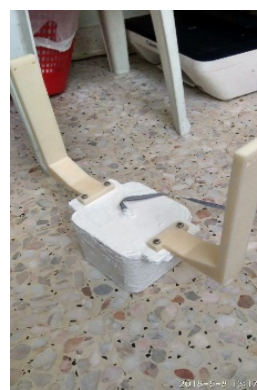
Fig. 6 — Pixy sensor pressure housing with supportive arms
